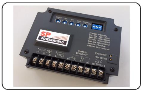
Engine Start Smoke Limiting function & IDLE Speed Setting For External, Built-in, PT-Pump type and hydraulic drive actuators Newly added "extreme slow response" engine setting
