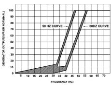
Figure 1 Frequency Compensation Curves
