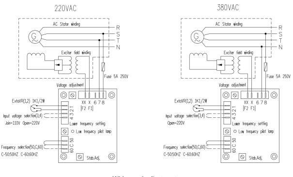
Wiring and adjustment Figure 4
