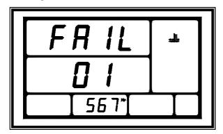
The [FAIL] and [01] represent the failure event log entry (01 to 15), [567Hr] represents the operating hour when the failure event occurred and the Coolant Overheat failure signal icon represents the cause of failure.
