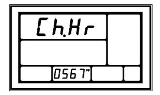
User can press [INCREASE] and [DECREASE] keys to change the stored value. By holding onto the increase and decrease keys can increase the speed of changing value to the desired value faster.
