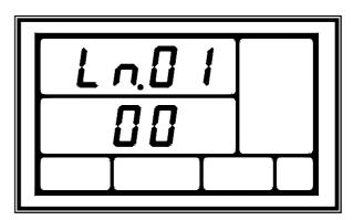
[ Ln.01 ] represents Setting entry No.1, [ 00 ] representing the entered value. User can press [ INCREASE ] and [ DECREASE ] keys to change the setting value. Each time when press [ SET ] key the current setting entry will move onto the next entry. If the setting is left unattended for 30 seconds or if the last entry have been completed the display screen will display [ End. ] message, meaning the system setting has been successfully completed and all modified value will be saved.
