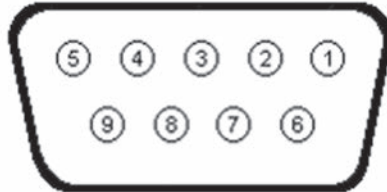
Figure 5-6. RS-232 Communication Port Terminal Positions
