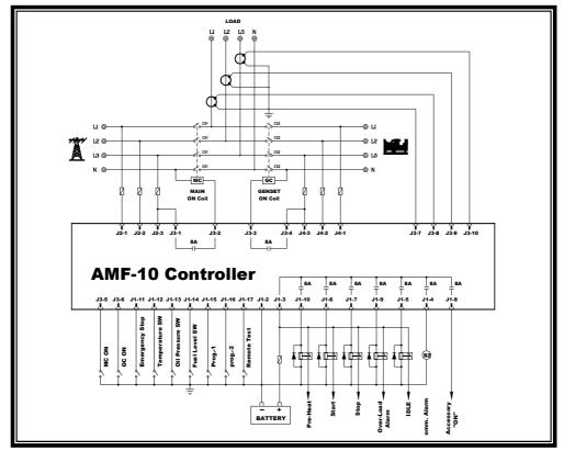
6.2.2 3 Phase 3 Wires Wiring Diagram
