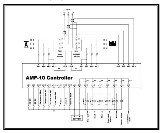
6.2.3 Single Phase 3 Wires Wiring Diagram
