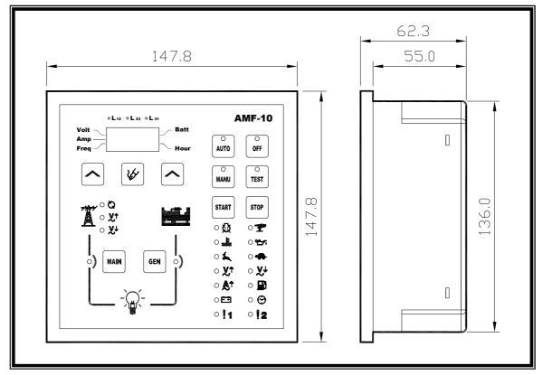
1.4 Panel Cut-out (Measurement : mm)
